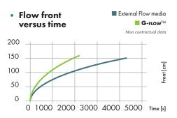
Comparison with 7 layers NCF 0/90 + External flow media versus 6 layers NCF 0/90 + G-Flow in internal position (3500gsm for each laminate)
